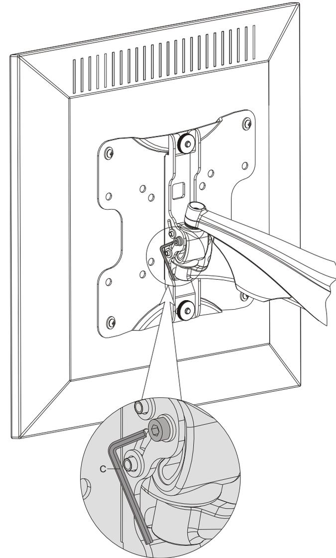
Depending on the weight of the display, it is necessary to slightly loosen or tighten the adjustment screw using an Allen key.
